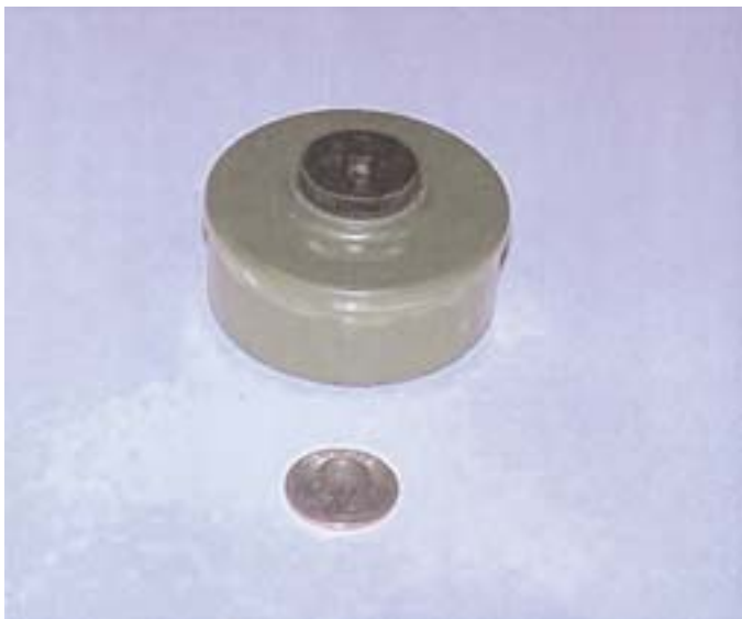
FIG. 1—PMA-2 anti-personnel mine casing.
